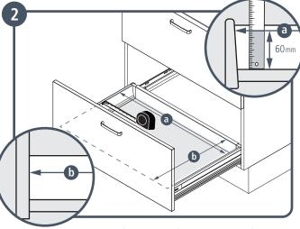
Measure 60mm up from the base of the drawer and carefully measure the inside width a and measure the inside drawer depth b.
