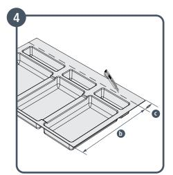
Carefully trim the tray depth according to the measurement **b**. Trim from the back edge **c** as needed.
