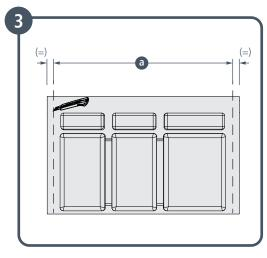
Carefully trim the tray width according to the measurement **a**.
