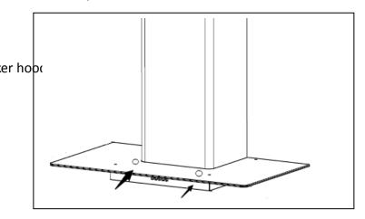
Fix the one-way-valve to the air outlet of the cooker hood. Then, attach the exhaust pipe onto the one-way-valve as shown below.
