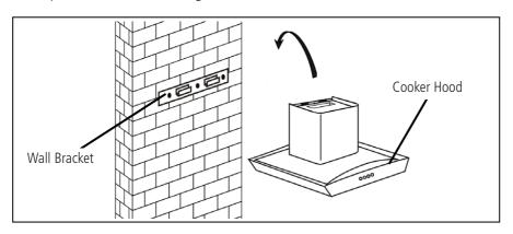
After hanging the hood on the bracket, remove the grease filters, mark 2 holes inside the hood for safety screws. After marking, remove the hood, drill two holes and insert 2 wall plugs and finally fix the safety screws with 2 screws (ST4x30mm).
