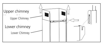
require is reached, attach the fixing hole to the f Assemble the side the chimney to adjust the chimney height. When the height would have been and drill the fixing hole and fix the upper chimney bracket with army lspheyws rats 2 strown ST4x30mm.
