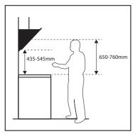
The cooker hood should be installed so that there is a space of 650-760mm from the centre of the mesh grease filters to the hob (435-545mm from the bottom of the hood to the hob). It is the manufacturer of the hob who determines the clearance required and the clearance quoted by the hob manufacturer must be followed. In the absence of any instructions supplied with a gas hob the minimum distance between the hob and the centre of the mesh grease filters must be at least 760mm.
