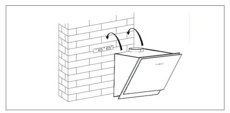
After hanging the hood on the bracket, remove the grease filters, mark 2 holes inside the hood for safety screws. After marking, remove the hood, drill two holes and insert 2 wall plugs and finally fix the safety screws with 2 screws (ST4x30mm).
