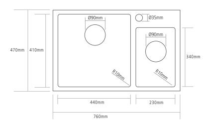
Bowl depth: 220mm Small bowl depth: 200mm Min. base unit: 800mm
