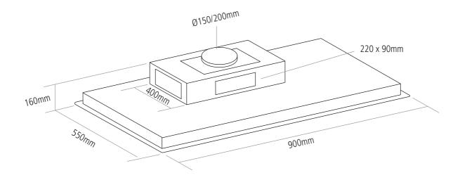
For installation into the ceiling a niche of 815mm x 515mm is required, with a minimum height of 170mm
