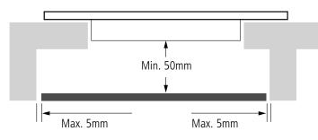
There are ventilation holes around the outside of the hob. YOU MUST ensure these holes are not blocked by the worktop when you place the hob in position.
