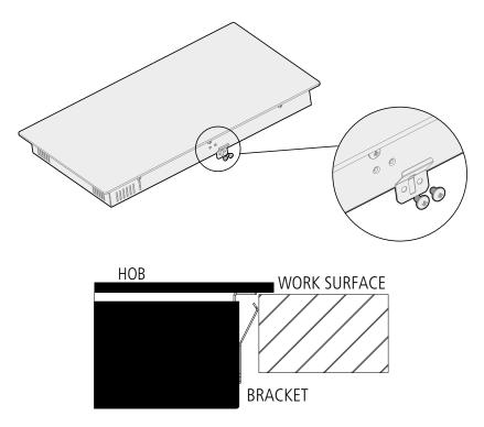
Under any circumstances, the brackets cannot touch with the inner surfaces of the worktop after installation [see picture]. This will ensure the hob is properly secured to the underside of the work surface.
