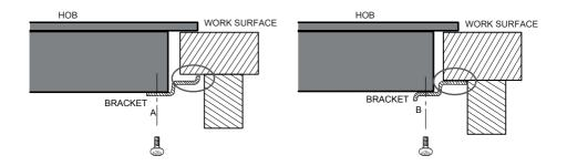
Under any circumstances, the brackets cannot touch with the inner surfaces of the worktop after installation [see picture]. This will ensure the hob is properly secured to the underside of the work surface.
