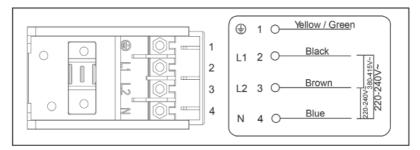
The appliance can be connected directly to the mains by single-phase electrical connection, as shown below.
