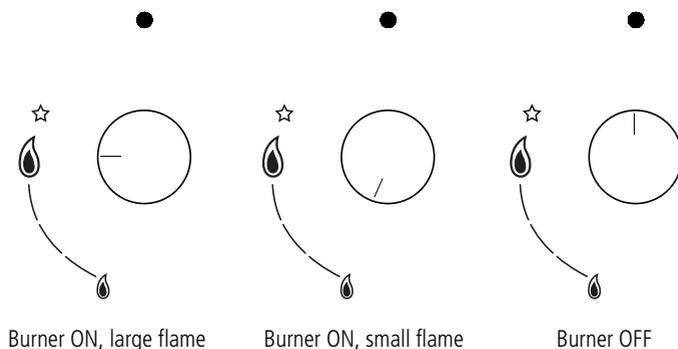
The burner should be set at a large flame during the initial phase of cooking to bring the food to boiling, and then the knob should be turned to the small flame position to maintain the cooking. It is also possible to adjust the flame size in smaller adjustments.
