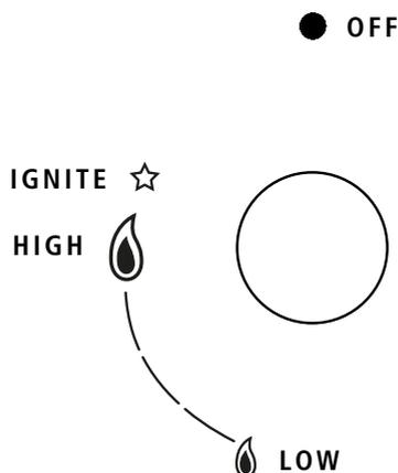
This hob is equipped with an ignition switch incorporated into the control knob. To light a burner, simply press the corresponding knob all the way in and, then, turn it in the counter-clockwise direction to the High setting, keeping it pressed in until the burner lights.
