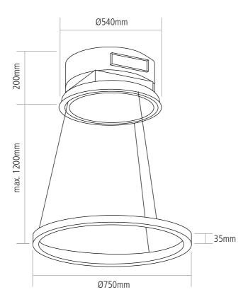
For installation create a false ceiling with a round niche of 510mm, with minimum height of 220mm.
