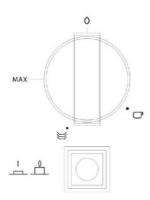
The control elements are the temperature knob and the luminous ON-OFF switch. With the switch pressed (position 1) the drawer is on, whereas when the switch is released (position 0) the drawer is off. These parts can be seen only when the drawer is open. When the drawer is closed, a control light located on the front of the appliance lets you see whether the drawer is on.
