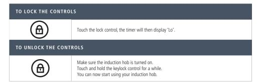
When the hob is in the lock mode, all the controls are disabled except the ON/OFF button, you can always turn the induction hob off with the ON/OFF control in an emergency, but you will need to unlock the hob first before the next operation.
