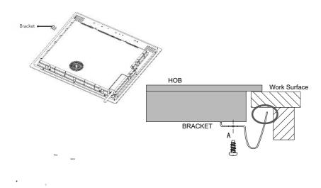
Under any circumstances, the brackets cannot touch with the inner surfaces of the worktop after installation (see picture). This will ensure the hob is properly secured to the underside of the work surface.
