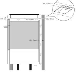
The panels of the adjoining furniture should be heat resistant. Particularly when the adjoining furniture is made of veneered wood, the adhesives should be able to withstand a temperature of 150°C. Plastic materials or adhesive which cannot withstand this temperature may become deformed or unstuck.
