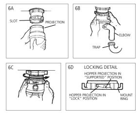
» If mount ring is hard to turn, you may add a small amount of petroleum jelly or liquid soap to hopper projections. Run water and check for leaks.
