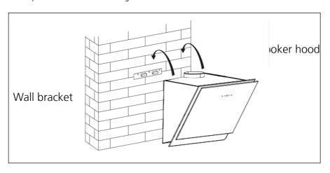
After hanging the hood on the bracket, remove the grease filters, mark 2 holes inside the hood for safety screws. After marking, remove the hood, drill two holes and insert 2 wall plugs and finally fix the safety screws with 2 screws (ST4x30mm).
