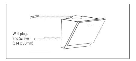
Place the plastic duct on the cooker hood outlet.
