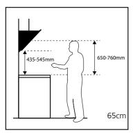
The cooker hood should be installed so that there is a space
