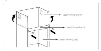
Putpther chimmeyon the cooker hood. Fix the lower chimney bracket on the wall by 2 screws (4mm x 30mm).
