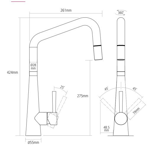
Worktop cut-out 35mm required Note: Pull-out hose extended by 400mm
