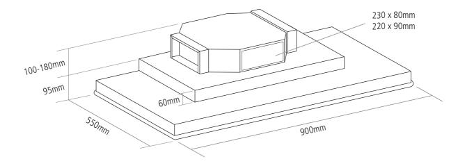
For installation into the ceiling a niche of 865mm by 515mm is required, with a minimum height of 200mm.
