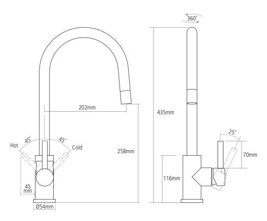
Worktop cut-out 35mm required Note: Pull-out hose extended by 500mm
