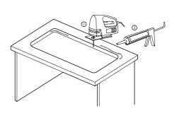
Cut a hole in the worktop following this second inner line. Alternatively use the template provided with the sink.
