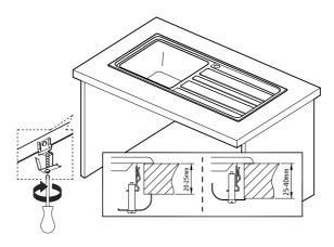
Using the fixing clips provided, secure the sink to the worktop by clipping these into the brackets under the sink, and screwing until the clip is tight against the worktop as shown.
