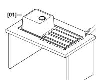
Place the sink upside down in the position where it is to be installed, and trace the outline of the sink on the worktop with a pencil.
