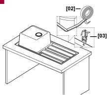
Apply the seal tape around the under side of the edge of the sink, being careful to lay it smoothly.
