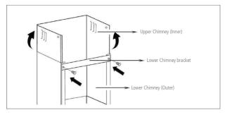
Putputer chimmeyon the cooker hood. Fix the lower chimney bracket on the wall by 2 screws (4mm x 30mm).
