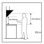
The cooker hood should be placed at a minimum distance of 650~760mm above the hob. It is the manufacturer of the hob who determines the clearance required and the clearance quoted by the hob manufacturer must be followed. In the absence of any instructions supplied with a gas hob the minimum distance between the hob and the hood must be at least 760mm.
