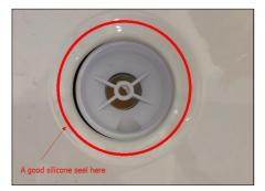
The image above shows the location of the required seal, it is important that an ample amount of sealant is used to ensure there are no small air bubbles or gaps which could allow a small amount of water to trickle through.
