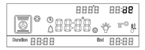
In demo mode, the normal operation of the cooling fan, circulation fan, and lighting work normally, however all heating elements and other functions are disabled.
