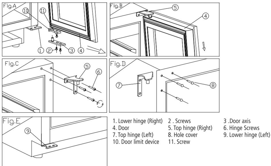
1. Open the door to a 90 degrees angle, take out the 2 screws (2) from lower door axis (3), remove the door (4), Remove the axis plate (3) from the door, (Fig. A).
