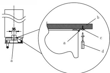
After installing the wine cabinet, please open the door, adjust the fixing bracket (a) and fix this in position with three screws (c) using a screwdriver (d) into the work surface (b).
