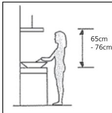
The cooker hood should be placed at a minimum distance of 65~76cm above the hob. It is the manufacturer of the hob who determines the clearance required and the clearance quoted by the hob manufacturer must be followed. In the absence of any instructions supplied with a gas hob the minimum distance between the hob and the hood must be at least 760mm.
