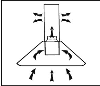
If you do not have an outlet to the outside, the exhaust pipe is not required (as shown in the section “Installation - ducted”), and charcoal filters must be installed.
