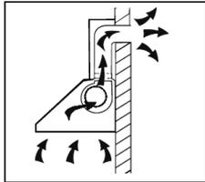
If you have an outlet to the outside, your cooker hood can be connected as per the below picture by means of an extraction duct with an interior diameter of 150mm.
