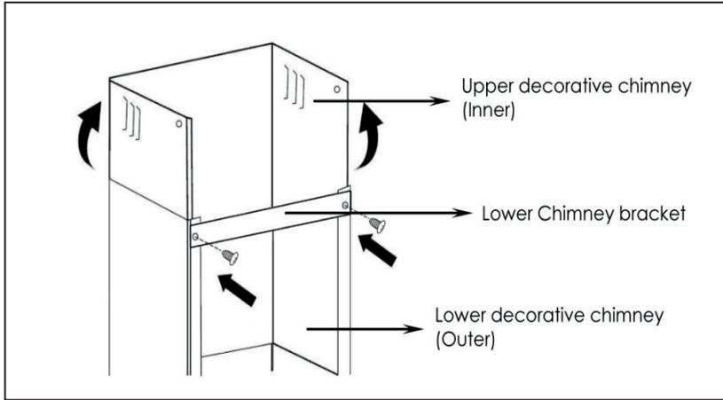
Drill 2x8mm holes to accommodate the plate II. Screw and tighten the plate II onto the wall with two screws and wall plugs provided. Slide up the upper chimney and fix the upper chimney with plate II with 2 screws ST4x8mm.
