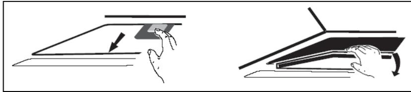
Fit the activated charcoal filter onto the side of the motor and turn it in a clockwise direction to lock into place. Repeat the same on the other side.
