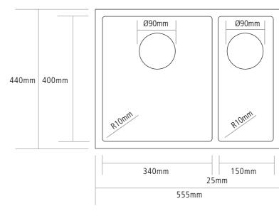
Bowl depth: 200mm Small bowl depth: 135mm Min. base unit: 600mm
