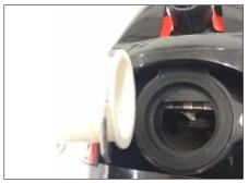
**WARNING:** This is an incorrect fitting, the joint will never be water tight.
