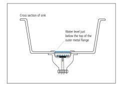
3. We will now explain exactly what the problem is. Basically, if water is draining away, but not through the plug seal, the sink has not been fitted correctly. The water is actually leaking underneath the metal flange due to a missing waterproof seal. In many cases, the installer has either dry fitted the metal flange providing no watertight seal between the metal flange and the ceramic sink. Or it is possible that the installer has used a fabric or rubber seal that is not adequate.
