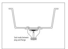
2. Push the sink plug down as you would normally to seal and then fill to just over the top of the plug with water. Be careful NOT to put too much water in. You do not want water to go over the top of the metal outer flange and into the sink. If the rubber seal on the plug is faulty, the water will now drain away and you will need to order a new plug. If the seal is not faulty the water will remain and, therefore, prove that there is nothing wrong with the plug.
