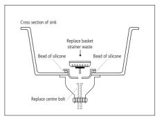
Leave the sealant to completely dry (please refer to the manufacturer's recommendations). Once dry you can put the plug back into position. Fill the sink up with water and you should find it no longer drains away.
