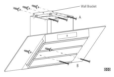
After hanging the ho**diation** the bracket, open the front panel and remove the grease filters, mark 2 holes inside the hood for safety screws. After marking, remove the hood, drill two holes and insert 2 wall plugs. Hang the hood back onto the wall and finally fix the safety screws with 2 screws (ST4x30mm) (B).
