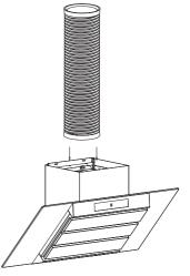
The upper chimney section sits inside the lower chimney section.
