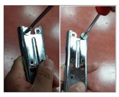
9. Screw the bottom hinge to the left bottom side of refrigerator. Screw the adjustable foot there.
