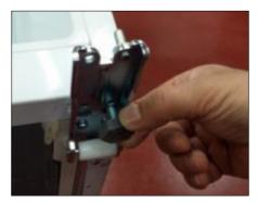
7. Unscrew the bottom hinge screws.
