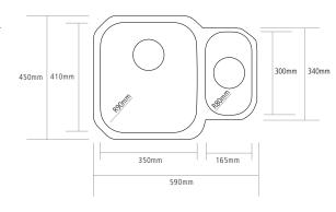
BOWL DEPTH: 180MM SMALL BOWL DEPTH: 125MM MIN. BASE UNIT: 600MM
