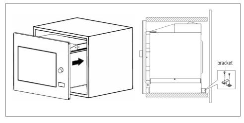
Open the door, fix the microwave oven to the cabinet with Screw B at the installation hole. Then fix the Trim-kit plastic cover to the installation hole.
