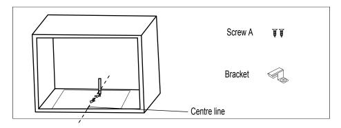
Remove the bottom cabinet template and fix the bracket with screw A.
