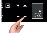
Set the clock with the + and - buttons: during setting the separator dots flash, the time has been set when the dots remain steady on.
