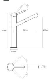
Note: Pull-out hose extended by 650mm Worktop cut out 35mm required
