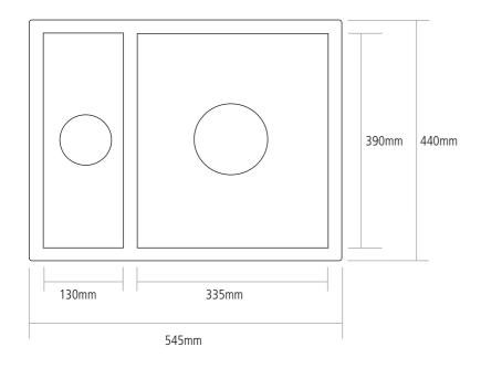
MAIN BOWL DEPTH: 178MM SMALL BOWL DEPTH: 118MM OVERALL SINK DEPTH: 200MM
