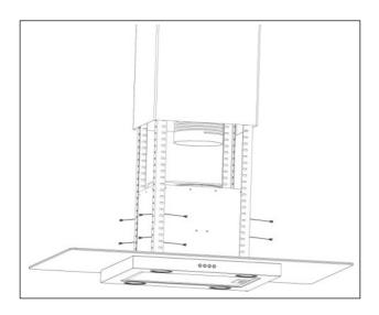
If you are using the hood in ducted / ventilation mode, you should fix e ducting hose to the ceiling.
