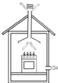
IN A CHIMNEY STACK OR BRANCHED FLUE
