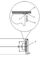
After installing the wine cabinet, please open the door, adjust the fixing bracket (a) and fix this in position with three screws (c) using a screwdriver (d) into the work surface.
