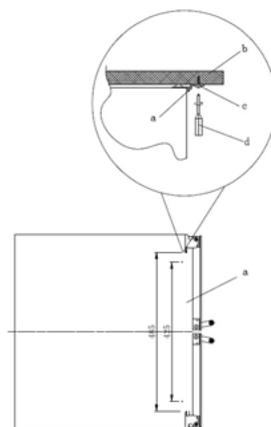
After installing the wine cabinet, please open the door, adjust the fixing bracket (a) and fix this in position with three screws (c) using a screwdriver (d) into the work surface (b).
