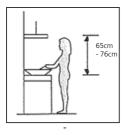
The cooker hood should be placed at a minimum distance of 65-76cm above the hob. It is the manufacturer of the hob who determines the clearance required and the clearance quoted by the hob manufacturer must be followed. In the absence of any instructions supplied with a gas hob the minimum distance between the hob and the hood must be at least 760mm.
