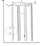
4. If your cooker hood is going to be externally ventilated, then you should connect the ducting hose to the ceiling adaptor at this point. Fix the upper chimney section to the hanging plate, using the 4 x self tapping screws.
