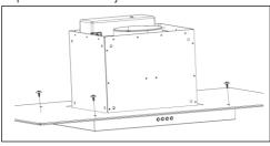
6. Lift the main body of the cooker hood onto the angle bars and then fix it into position using the 16 x M5 screws.
