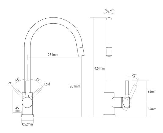
Worktop cut-out 35mm required Note: Pull-out hose extended by 650mm
