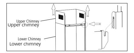
Slide the chimney to adjust the chimney height. When the height you require is reached, mark and drill the fixing hole and fix the upper chimney bracket with 2 wall plugs and 2 ST4x30mm.
