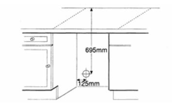
If the through the wall vent is to be positioned other than behind the dryer, the vent hose should be positioned at floor level and through adjacent side panel to a relevant position. The plinth must be cut-out to accommodate the air vent grill at the bottom front of the tumble dryer.
