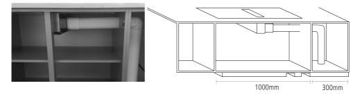
If you choose to run the ducting inside the cabinet directly below the hob, you can still achieve the use of full depth drawers and full width drawer fronts by installing a divider inside the main carcase as pictured below (the drawer boxes must be reduced in width to allow for the divider):
