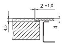
The outside dimension of the recess should always be about 6 mm longer than the outside dimension of the glass ceramic hob so that a seal can be provided (see: "Gluing in the hob").
