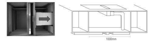
You can then use the supplied ducting sections to connect to the motor in the most suitable location. There are various options including going straight down in the below cabinet or extending the duct channel to the right into an adjacent 300mm cabinet, which can house the round 150mm tube. The latter method allows the most use in the cabinet below the hob as the main part of the ducting is housed in a 300mm wide cabinet to the right of the product.
