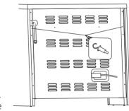
The cooker is supplied with an anti-tilting chain to prevent the appliance from tilting forward and causing accidental damage to the gas pipe. Make a hole in the wall behind, at the same height as the fixing chain. Insert the plug into the hole and then screw in the hook until it is firmly fixed to the wall. Fix the chain to the hook. You can adjust to level of the cooker by inserting the feet provided.
