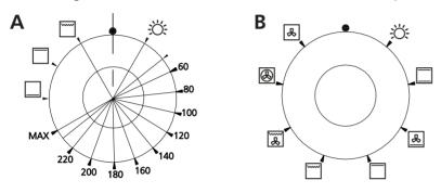
Control A is for cooking temperature selection, control B is used to select the required function.
