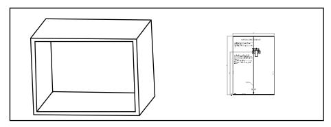
2. Make the marks on the bottom plane of cabinet according to marks "a" on the template
