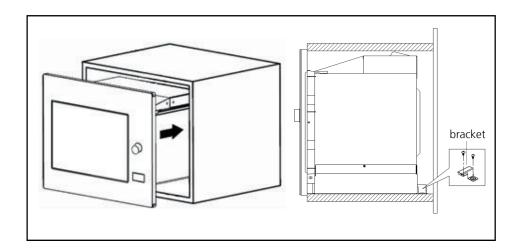
5. Open the door, fix the oven to the cabinet with Screw B, at the installation hole.
