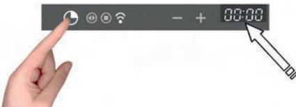
The separator dots flash to indicate you can set the time.
