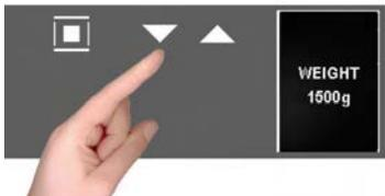
The weight screen appears. Use the ▼ ▲ buttons to select the preset values and confirm the choice with the □ button.
