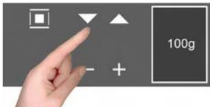
After you have selected the dish with **▼ ▲** and confirmed with **■** the display shows the weight to set, starting from an initial minimum of 50 g; using **▼ ▲**, you can increase or decrease the weight and then confirm the choice with **■**.
