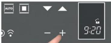
Set the clock with the + and - buttons: during setting the separator dots flash, the time has been set when the dots remain steady on.
