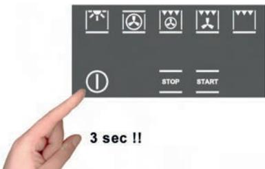
The key function is activated/deactivated by pressing the ① button for at least 3 seconds.
