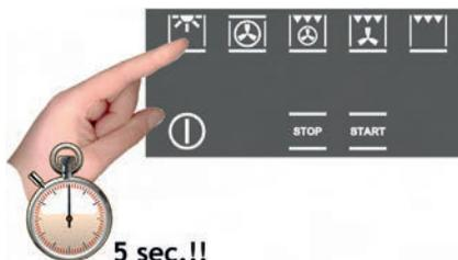
To disable the demonstration mode, touch the light symbol for five seconds: □ the control will go to normal operation and ready for turning on.
