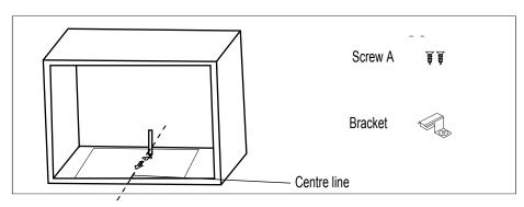
Remove the bottom cabinet template and fix the bracket with screw A.
