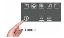
The key function is activated/deactivated by pressing the  $\bigcirc$  button for at least 3 seconds.
