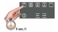
To disable the demonstration mode, touch the light symbol for five seconds: The control will go to normal operation and ready for turning on.
