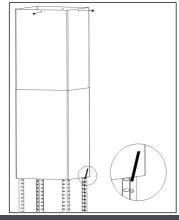
If the glass canopy has not been pre-assembled at the factory, then it should be fixed to the top of the main body of the cooker hood at this stage.
