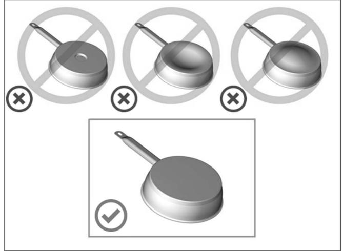
Do not use cookware with jagged edges or a curved base. To avoid scratching the glass, always lift pans off the hob - do not slide.
