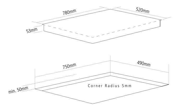
A minimum gap of 20mm is required beneath the hob fans, and a 4mm gap must be left under the worktop at the front of the hob for ventilation.
